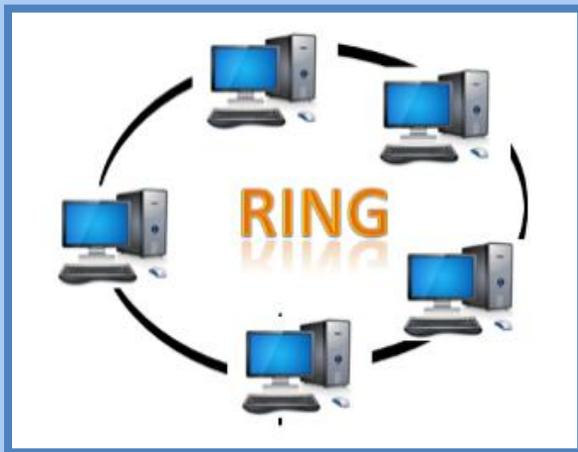
In ring topology the nodes are arranged in a circle (or ring). The data can travel through the ring network in either one direction or both directions, with each device having exactly two neighbours.
