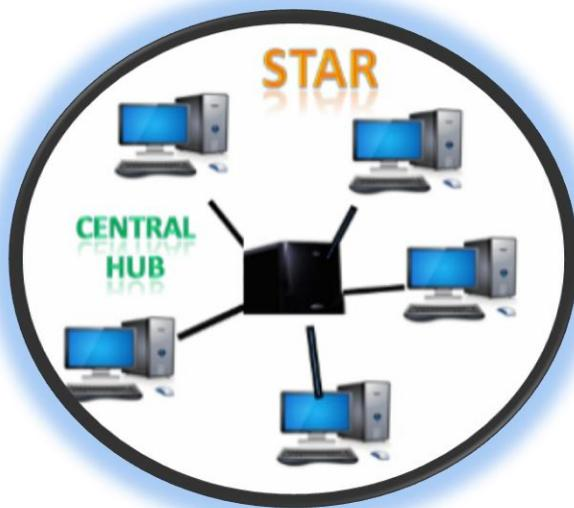
A star topology, the most common network topology, is laid out so every node in the network is directly connected to one central hub via coaxial, twisted-pair, or fiber-optic cable. Acting as a server, this central node manages data transmission—as information sent from any node on the network has to pass through the central one to reach its destination—and functions as a repeater, which helps prevent data loss.
