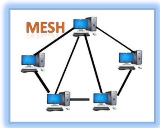
A mesh topology is a structure of point-to-point connections where the nodes are interconnected. Mesh networks can be full or partial mesh. Partial mesh topologies are mostly interconnected, with a few nodes with only two or three connections, while full-mesh topologies are fully interconnected. The web-like structure of mesh topologies offers two different methods of data transmission: routing and flooding.
