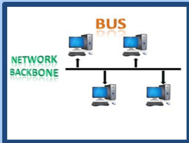
A bus topology connects all the devices on a network along a single cable running in a single direction from one end of the network to the other. It is sometimes called a line topology or backbone topology. Data flow on the network follows the route of the cable, moving in one direction.
